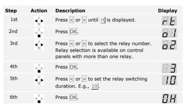
The relay switching duration was set. The system is in normal mode.
