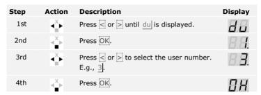
The user has been deleted. The system is in normal mode.
